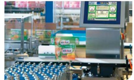
egrated checkweighing solutions ensure the completeness of assemblies, kits or individual delivery units. In filling systems, weighing is the only method of filling control that is not dependent on container shape, density differences, foam formation or air pockets.
